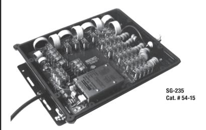
With a sophisticated Pi-L network and over 1/2 million tuning combinations, the SG-235 is the smartest way to tune at 500 Watts.
